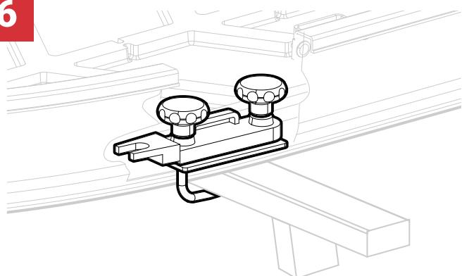
Ensure the roof top carrier is securely fastened to the cross rails.
