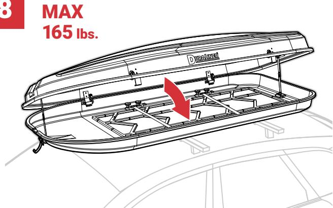
Evenly distribute luggage and gear within the roof top carrier. Lower the lid. Insert keys into locks, rotate horizontal and remove keys. Fasten front and rear draw latch.
