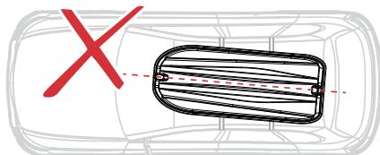
Ensure the roof top carrier is centered on the cross rails.
