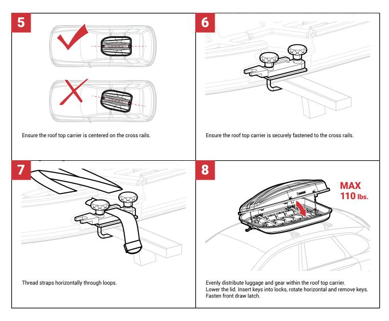
**WARNING:** The Duraliner Roof Top Carrier must be mounted securely to a roof rack with cross rails. Inspect mounting hardware periodically. Before each use, fasten the draw latch, and lock with keys.
