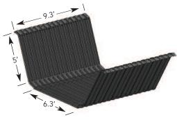
CAD rendering of typical MegaDitch 115° one base and one arm configuration. Each Sidewall Panel section is approximately 5'x9.3' Each Base Panel section is approximately 6.3'x9.3'
